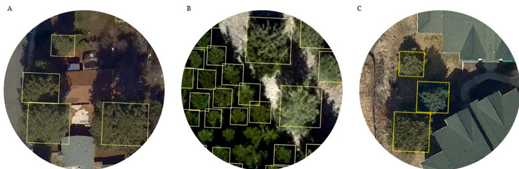
Fig. 6. Examples of detected tree crowns in Pullman under the (A) test dataset and different case studies: (B) high-dense tree canopy arrangement and (C) random tree arrangement close to buildings. A few trees were not detected in the clustered tree arrangement case study.
