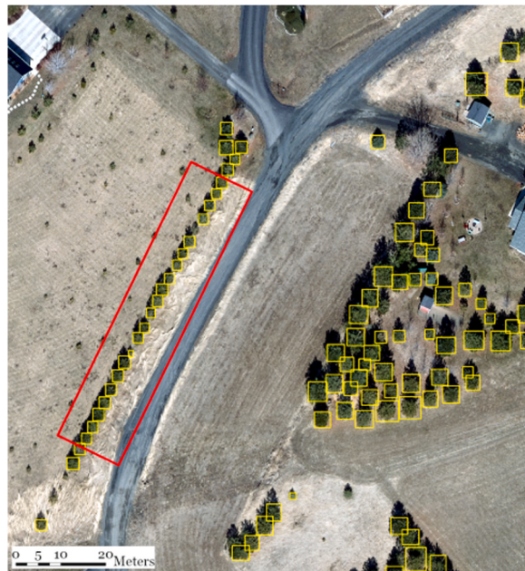
Fig. 9. Examples of small tree canopies detected in the study area based on the large-scale prediction using the PTCNet. The highlighted area (red rectangle) indicates small trees (<3m) with small tree crowns.
